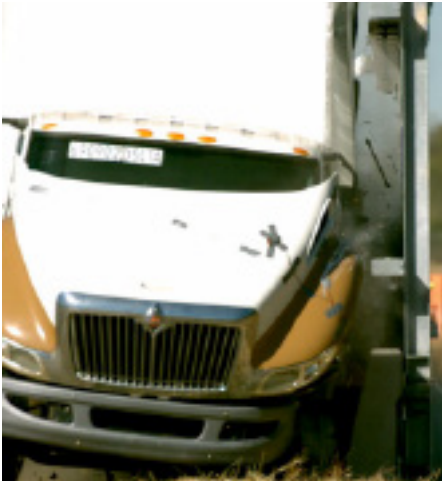
DAMAGED AREAS SHOW HOW THE SYSTEM REDUCES THE SEVERITY OF THE CRASH
