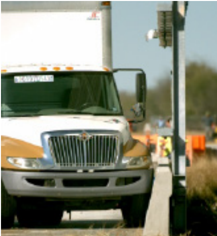
A 10,206 KG TRUCK IMPACTS THE MASH TL-4 SYSTEM AT 58MPH ON A 15° ANGLE
